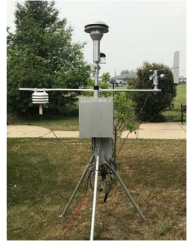
Figure 1: Photo of EBAM deployed for emergency response support monitoring.
